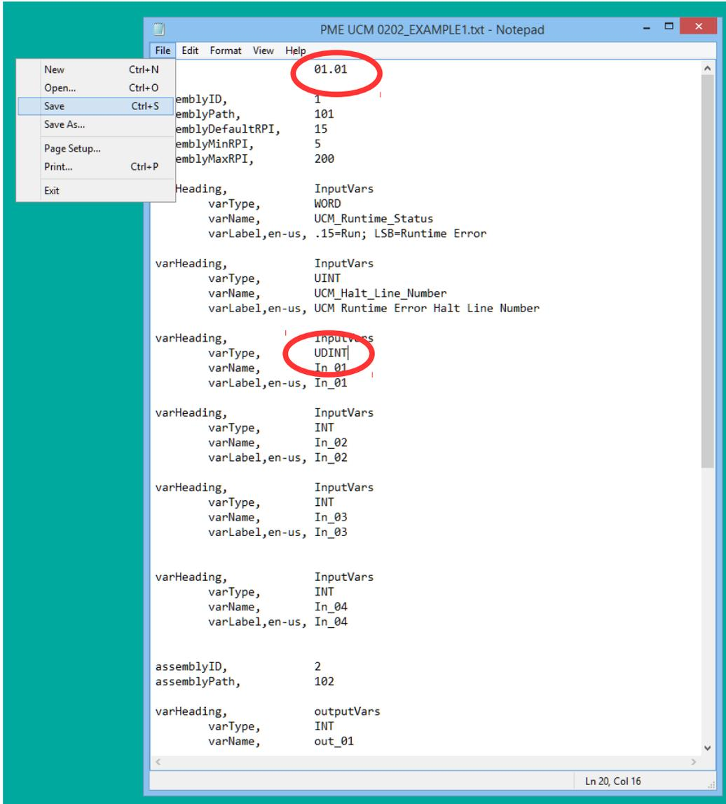
In this example, the SW version is changed from 1.00 to 1.01. Also, the varType of In\_01 is changed from an UINT to a UDINT. The new version is saved with the same filename.
