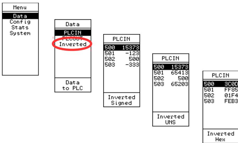
EDITABLE – The PLCIN data is set from the front panel of the PMEUCM.
