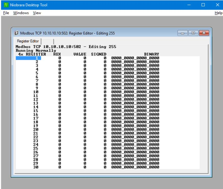
Typing in a value in the blue cursor enters the new value. Typing in 200 in the Register number will cause the viewer to jump to register 200.
