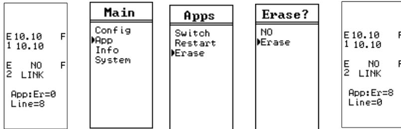
Notice that the App:Er=8 after the erase command is processed. Error 8 means that the checksum for the application is bad and the app will not run.
