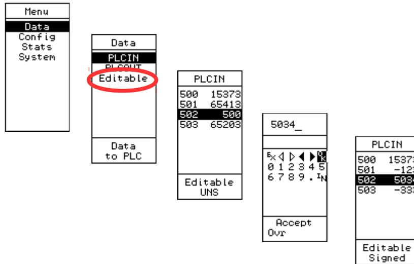
In this example, the value in register 502 is changed from 500 to 5034. Now the value in the M580 has changed to 5034 while the Out\_03 stays at -500.
