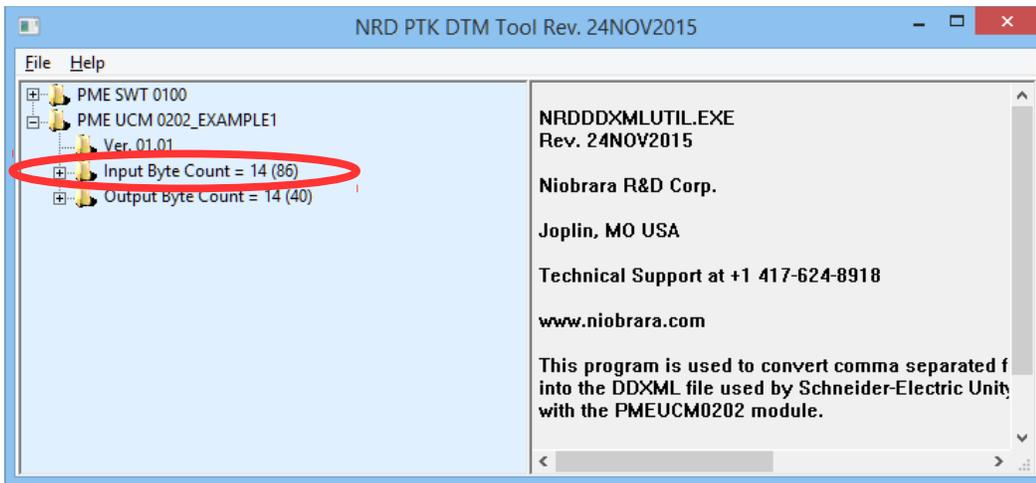
Expanding the tree shows the new structure for the PLC INPUT data:
