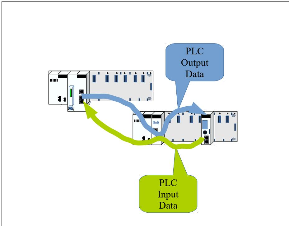
Each Ethernet/IP message from the CPU is transported via the RIO ring, through the CRA, and across the Ethernet backplane to the PMEUCM.
