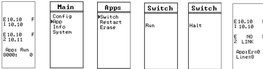
If all else fails, push the joystick “IN” for “Enter” and “UP” at the same time and hold for 10 seconds. This will cause the application to halt and exit to the OS.
