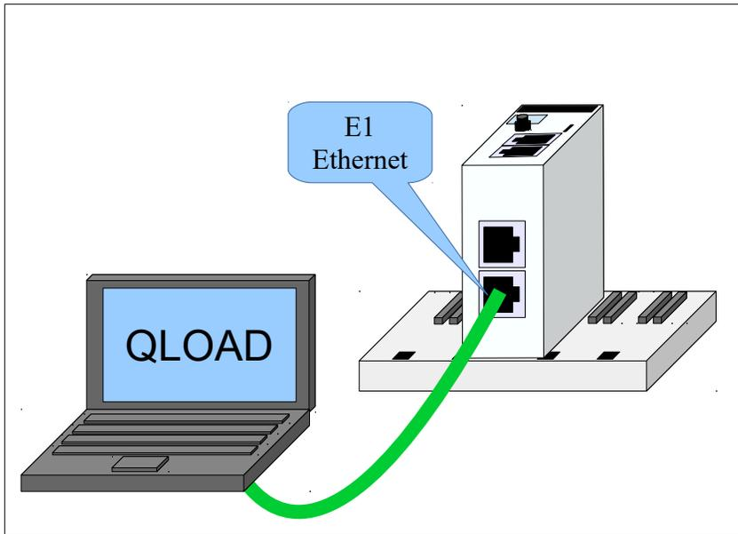
Connect the Ethernet port of the computer to E1 on the PMEUCM with a standard CAT5/6 cable.
