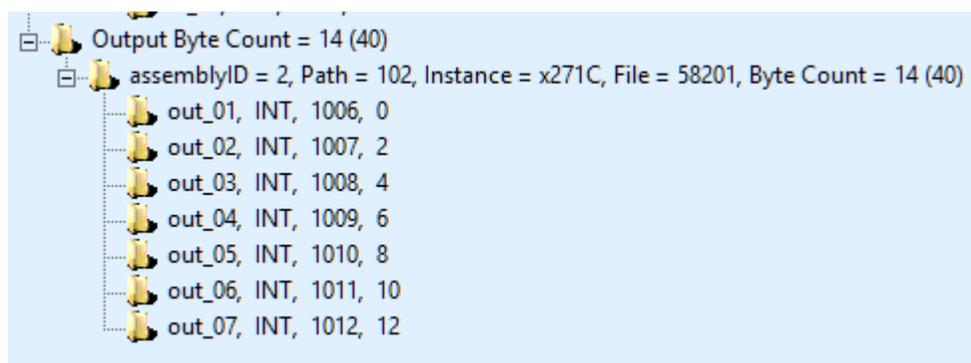
Again there is the byte count of outputs 14, followed by the total byte count including the PTK overhead of 26 bytes (40). The assemblyID = 2 and Path = 102 are from the .txt file. The Ethernet/IP index 1006 is next followed by the byte offset from the start of the data structure.
