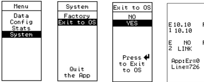
If the application does not include this type of screen driver but shows the OS screens, navigate to the Main > App > Switch > Halt screen.
