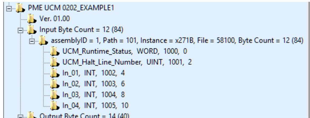
The heading shows the total number of bytes of PLC INPUT data. In this case there are 12 bytes of data. The number following (84) gives the total number of bytes including the PTK header information.
