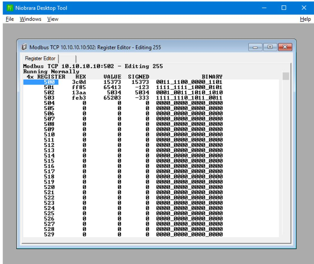
Notice that register 502 has the value 5034 that was entered from the front panel. Because the DATA configuration is still set for EDITABLE, we can manually enter data in this Modbus viewer and see the new data show up in the M580.
