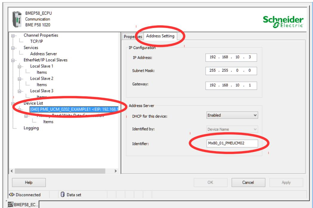
The “Identifier” must be modified to define the exact Rack and Slot occupied by
