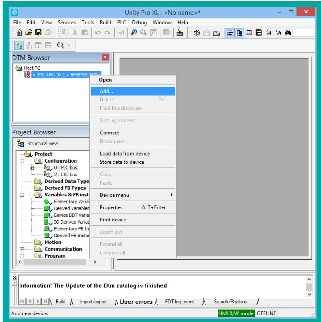
A window will pop up showing all of the installed DTMs. Scroll down until you reach the PME UCM 0202 EXAMPLE1 device by Niobrara.
