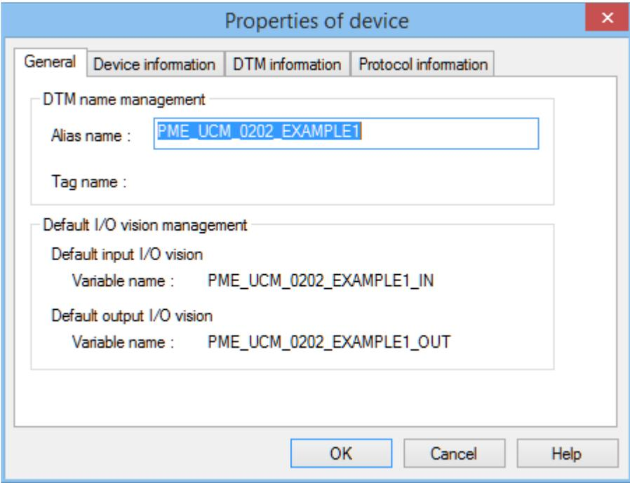
Pressing “OK” will add the DTM device to the DTM Browser.
