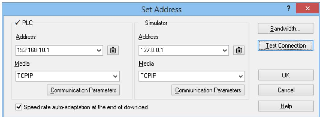
It is usually a good idea to try the “Test Connection” button to make sure that the PC can connect with the M580.
