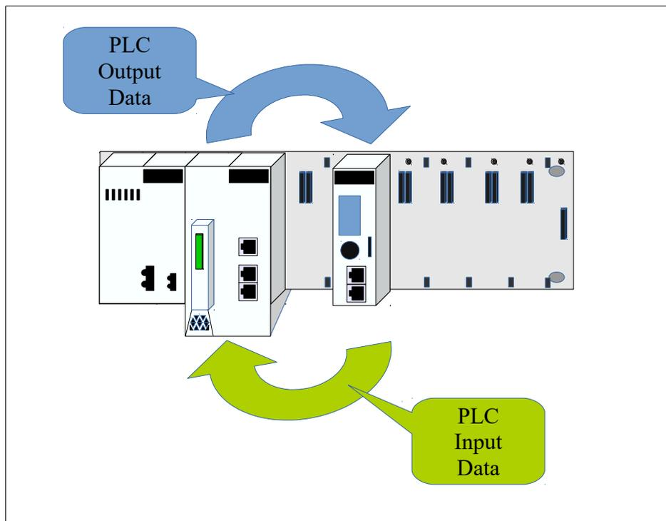
In the case of the PMEUCM located in an eRIO rack, the exchange happens across the RIO ring from the CPU through the CRA and across the Ethernet backplane to the PMEUCM backplane interface.
