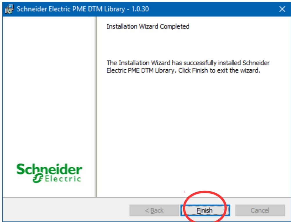
After selecting “Finish”, the S-E Wizard will close. Now close the PME\_TCM\_Libraray\_Setup window to complete the setup.
