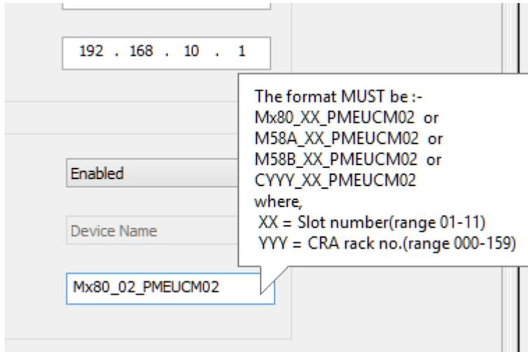
NOTE: If the PMEUCM is located in a remote rack, the YYY value is the thumbwheel (rotary switches) setting of the eCRA, not necessarily the logical rack number.
