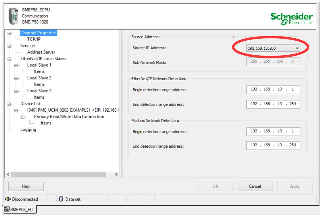
After Setting the Source IP Address, click on the PME\_UCM\_0202\_... entry in the list on the left.
