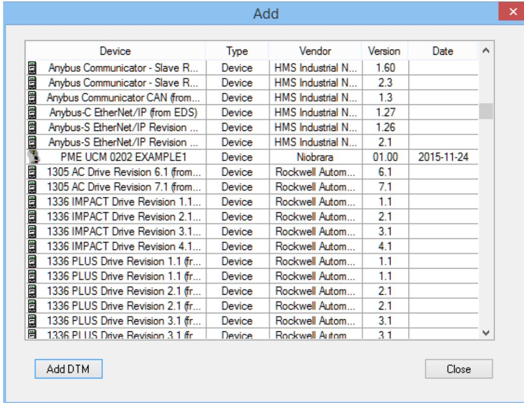
Press Enter or "Add DTM" to load the DTM for the PMEUCM. A window will pop up with information about the DTM.
