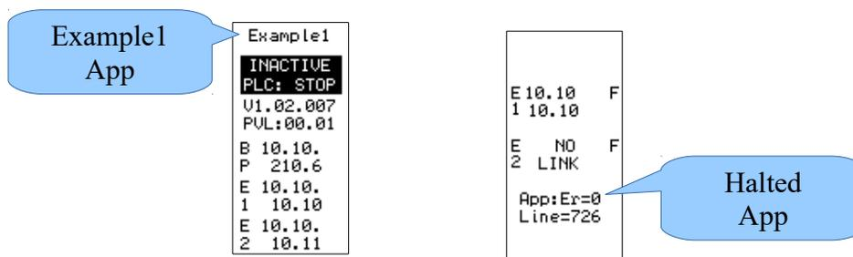
If the screen shows “Example1” at the top then the proper application is already loaded, but it is a good idea to qload a new copy anyway.
