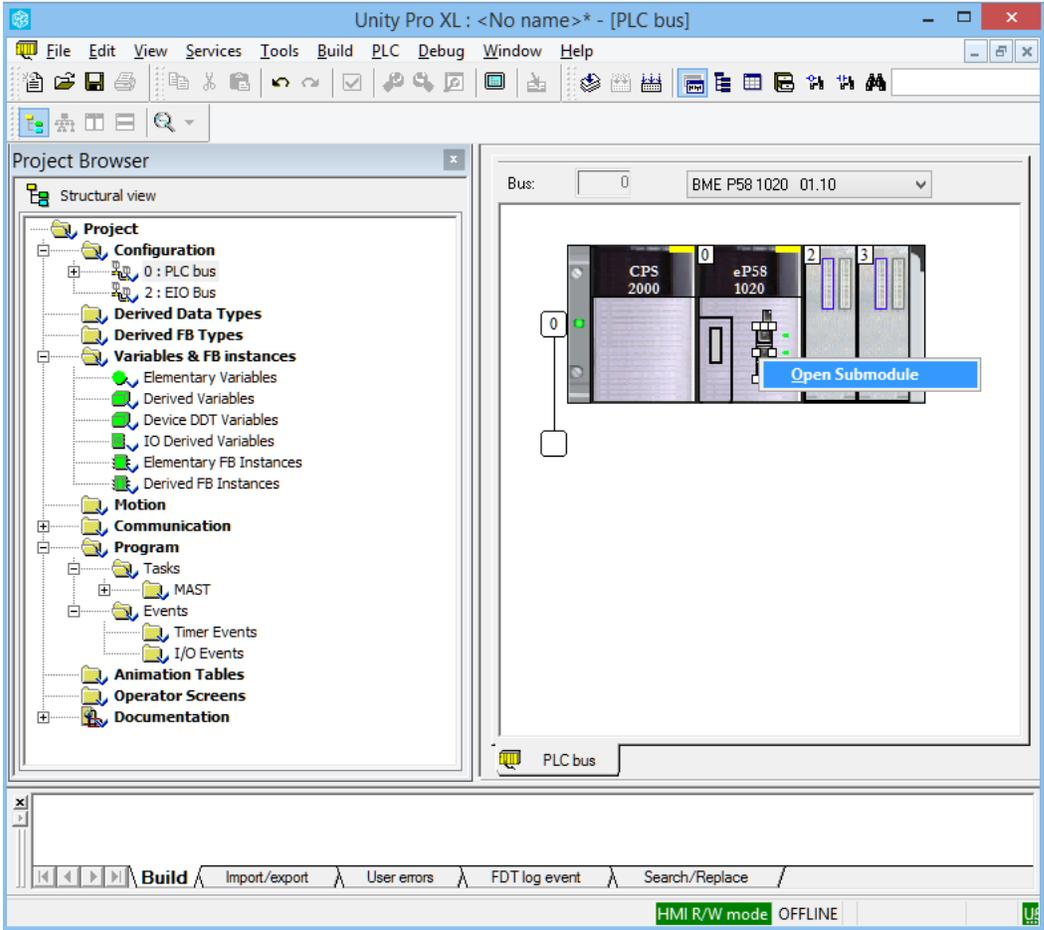
The FTP server must be enabled in the PLC for any PTK Partner module to function. The easy way to enable this server is to select “Unlock Security”.
