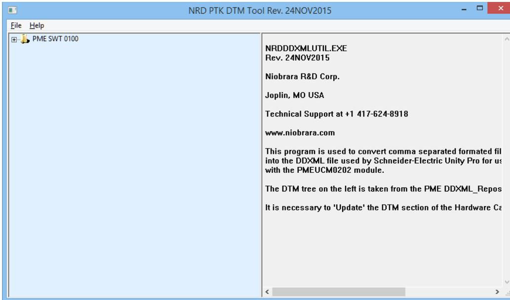
The tree on the left of the screen shows the PTK DTMs installed in Unity Pro. In this case, it shows the PME SWT 0100 Weighing Module from SCAIME.
