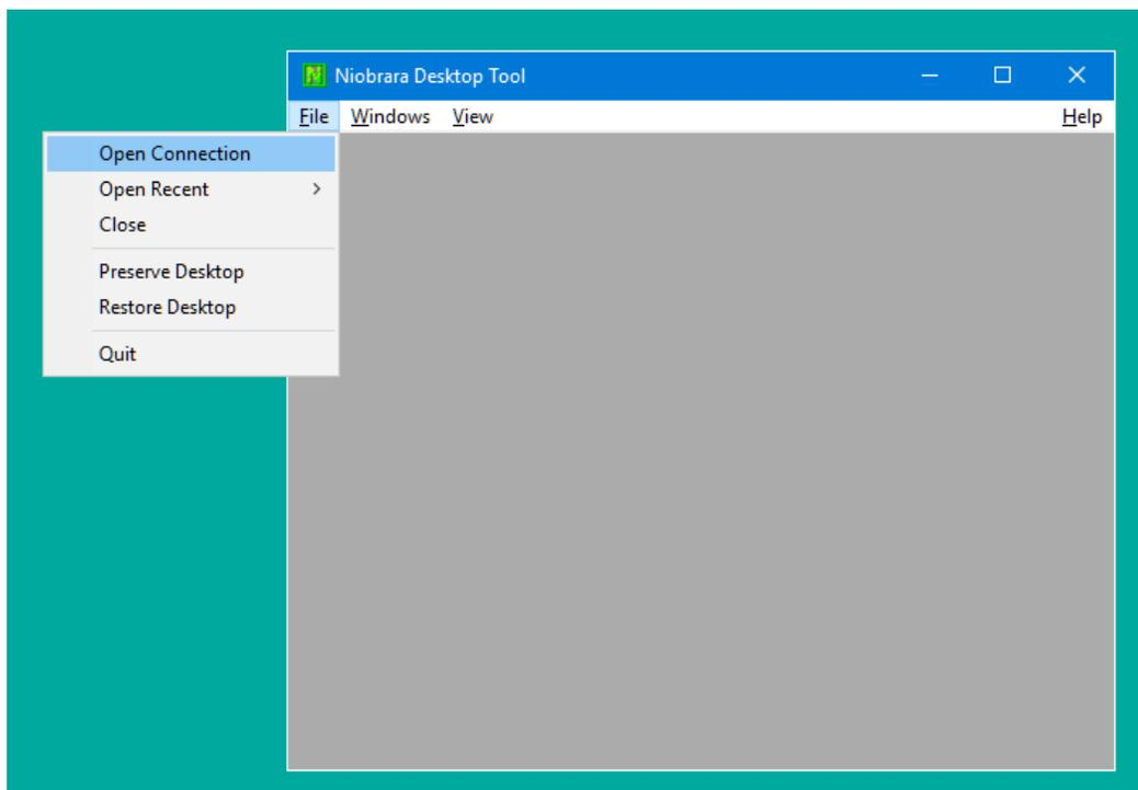
To open a new Modbus/TCP connection to the PMEUCM, Select File >Open Connection.
