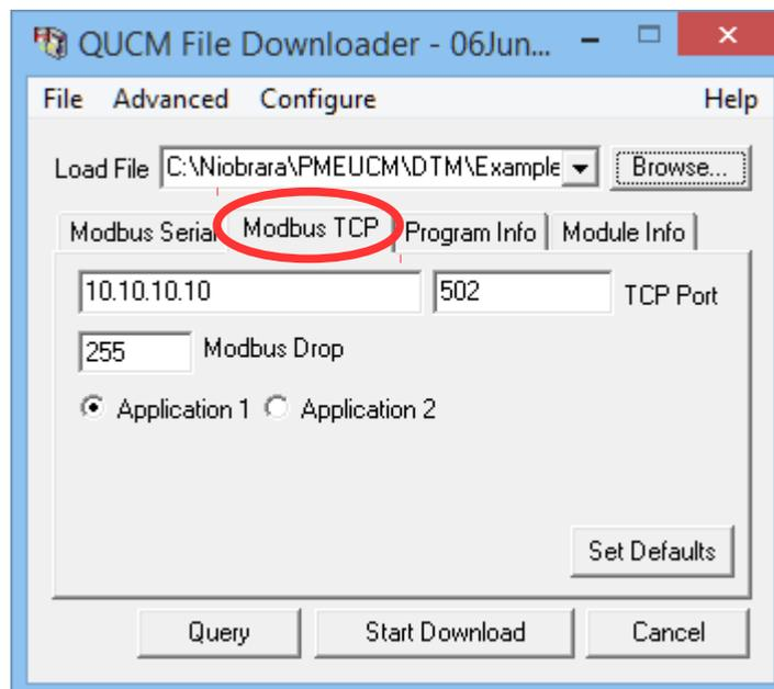
Make sure that the IP Address is set to match the PMEUCM E1 port of 10.10.10.10, the TCP Port is set to 502, Modbus Drop is 255, and Application 1 radio button is set.
