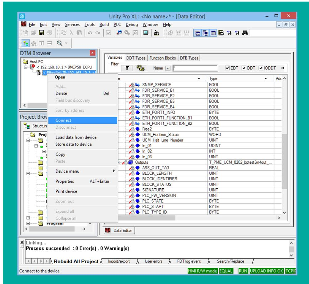
If the connection is successful you will be able to select: Device Menu > Additional Functions > Reset Device.
