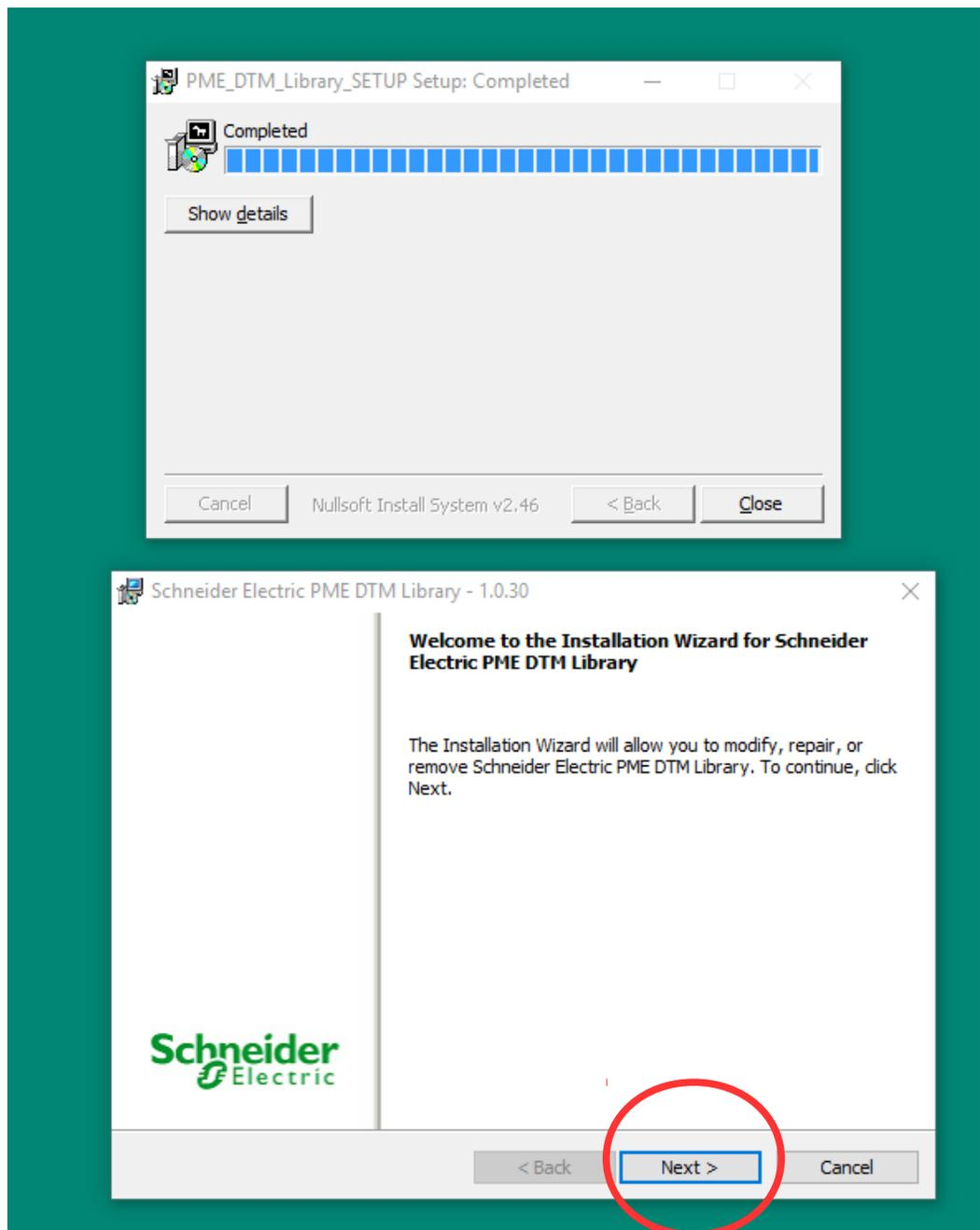
If you have a previous version of the PME DTM Library installed, you may be prompted to Repair or Remove the previous installation. Select Repair.
