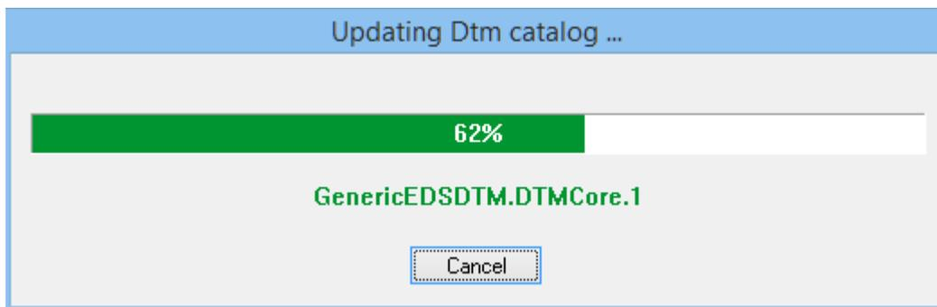
After the catalog update is complete, the new Niobrara DTM device should be listed in the hardware catalog. Also, the “User Errors” display should show “Information: The update of the Dtm catalog is finished”
