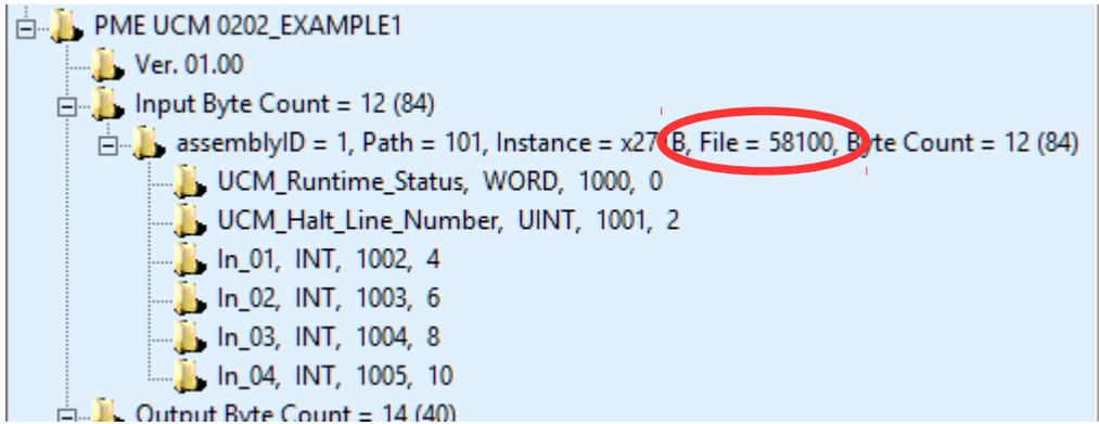
Also notice that the first 4 bytes of this file are the UCM Runtime Status and Halt Line Number. The UCM operating system automatically fills in these two values so the UCM application must start its data with an offset of 4 bytes as shown in the WRITE FILE line of code above.
