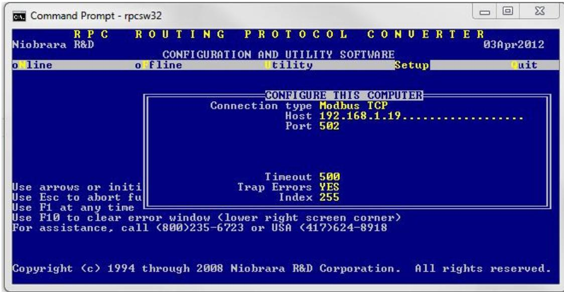
Figure 9.21 Setup Serial Screen for Modbus/TCP connection
