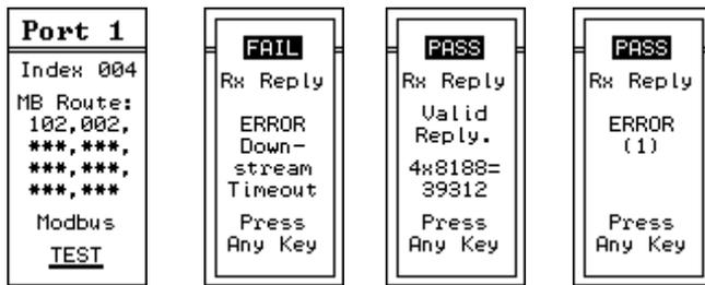
Figure 4.2 Modbus Route Edit TEST Screens
