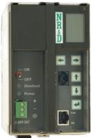
The CERI Module is a Compact Ethernet Remote Interface. It replaces the PLC CPU or DEA-202 interface in a Compact Primary Rack and maps the installed A120 I/O to Modbus/TCP. The CERI can then be controlled via Ethernet from another PLC with a standard I/O Scanner allowing a simple migration to the M340 while retaining existing racks and I/O. Device is configured through the built-in Web server and front panel LCD/keypad.
