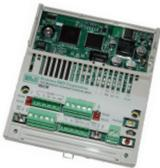
The MUCM is a user programmable serial communications Momentum specialty base that interfaces with Momentum communication adapters and PLCs. Two isolated RS-232 and/or RS-485 ports are provided. The MUCM is a powerful module that can be used in a variety of stand-alone applications such as serial protocol converter, data logger, or ASCII serial device interface.
