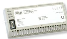
Niobrara's MST products are optically isolated serial communications adapters for TSX Momentum I/O. The MST may be used with any Momentum I/O Base to allow read+write control from a serial network. RS-485 and RS-232 versions are available with many common protocols including Modbus RTU and ASCII.
