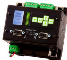
The MEBII is a new DIN rail mount version of the popular MEB-RT. It is a Unity Pro compatible, fully functional, bidirectional Modbus Plus (MB+) to Ethernet bridge. As a bridge, the MEBII routes data and PLC programming messages through all combinations of Ethernet, Serial RS-232/485, and MB+. Full bridging of programming messages from Unity Pro, Concept, and ProWORX is supported from Ethernet, MB+, and RS-232/485 serial.
