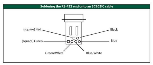
When all wires have been soldered, complete assembly by trapping slide locks and cable connector between halves of the supplied backshell and snapping together firmly. The SC902 is now ready for connection to the appropriate devices.
