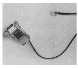
The MD422 is only used with a single Micro-1 processor. The RS-422 end features Square D® compatible slide locks like the CC-100 and the Micro-1 end has the same miniature modular connector as the FCB-15. The Micro-1 powers the MD422.
