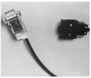
the CC-100 and the Model 50 end has the same connector as the FCB-10. Like the RIU-10, the ID422 includes an echo strap for normal operation of the CRM540 or some operator interfaces. The ID422 is powered by the Model 50. The device is available without the echo strap for special applications, order Niobrara part number **FA422.** Other Niobrara products provide Model-50 to RS-232 conversion (**SC50D** or **SC50I**), and Micro-1 to RS-232 (**SCM1D**) or RS-422 (**MD422**) interfaces.
