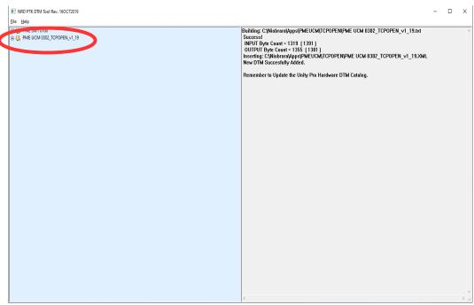
Clicking on the + will expand the TCPOPEN structure to show an overview of the PLC Inputs and Outputs.
