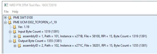
Expanding the Inputs reveals the variable passed from the UCM to the M580 CPU.
