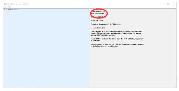
The tree on the left of the screen shows the PTK DTMs installed in Unity Pro. In this case, it shows the PME SWT 0100 Weighing Module from SCAIME.
