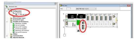
After selecting the "PLC Bus" in the Structural View Tree, double-click on the Ethernet ports of the CPU to open the configuration submodule.
