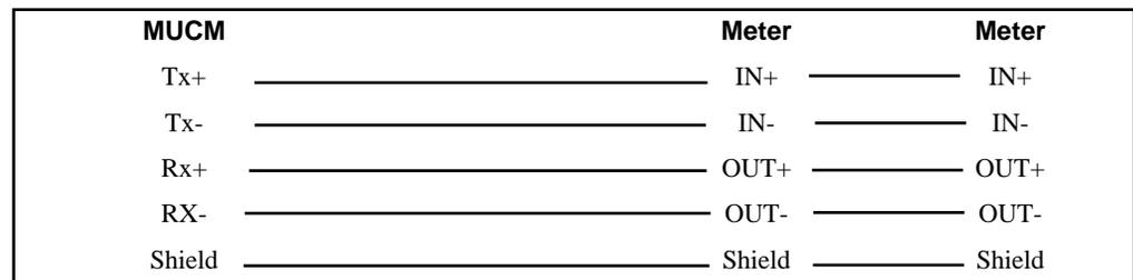
**Figure 2-4 MUCM to Powerlogic meters**
