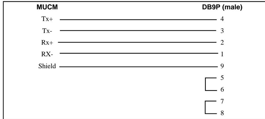
**Figure 2-3 MUCM to SY/MAX RS-422 port (MU7 Cable)**
