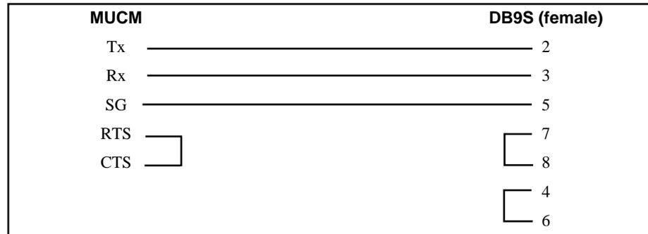
Figure 2-1 MUCM to PC RS-232 (MU1 Cable)
