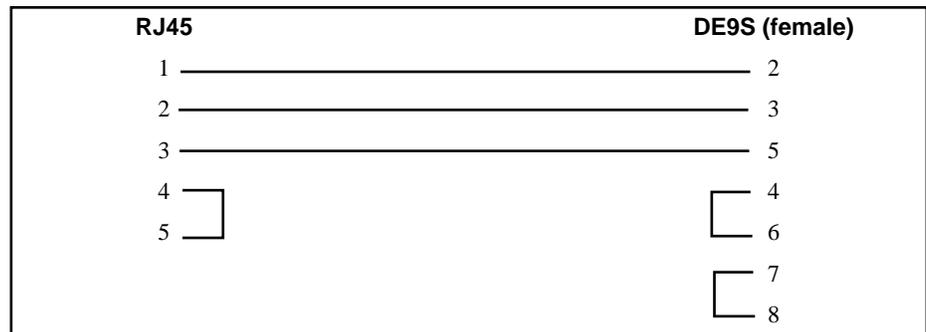
**Figure 2-4 MUCM to RS-232 PC DCE Port (9-pin) (MU1 Cable)**
