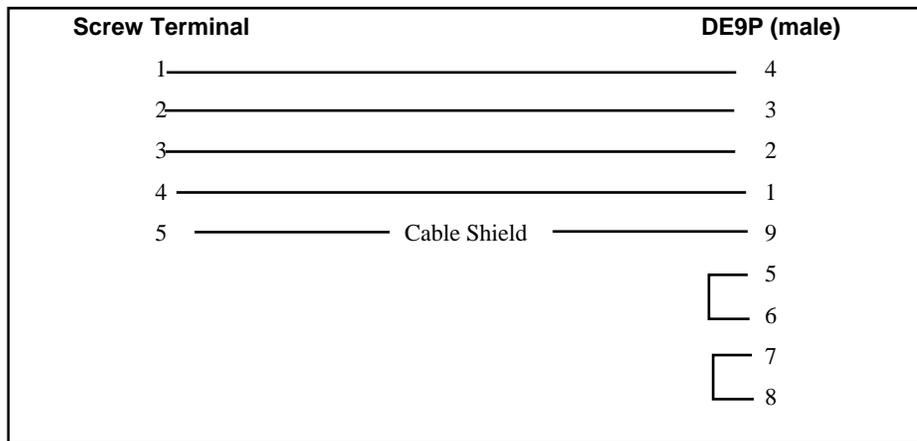
**Figure 2-2 RS-485 SY/MAX Port (9-pin) (MU7 Cable)**
