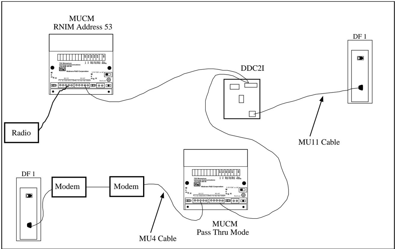
Figure 4-5 Pass Thru Example
