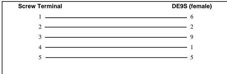
Figure 2-5 MUCM RS-422 to DF1/Data Highway Convertor RS-422
