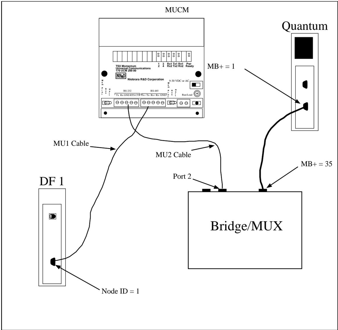
Figure 4-1 Modbus Plus Example
