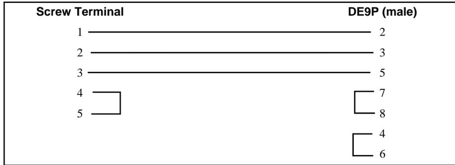
**Figure 2-1 MUCM to RS-232 DTE Port (9-pin) (MU2 Cable)**
