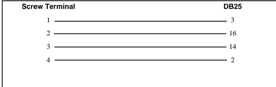
Figure 4-3 MUCM RS-422 to Helm Loadgard Serial Interface
