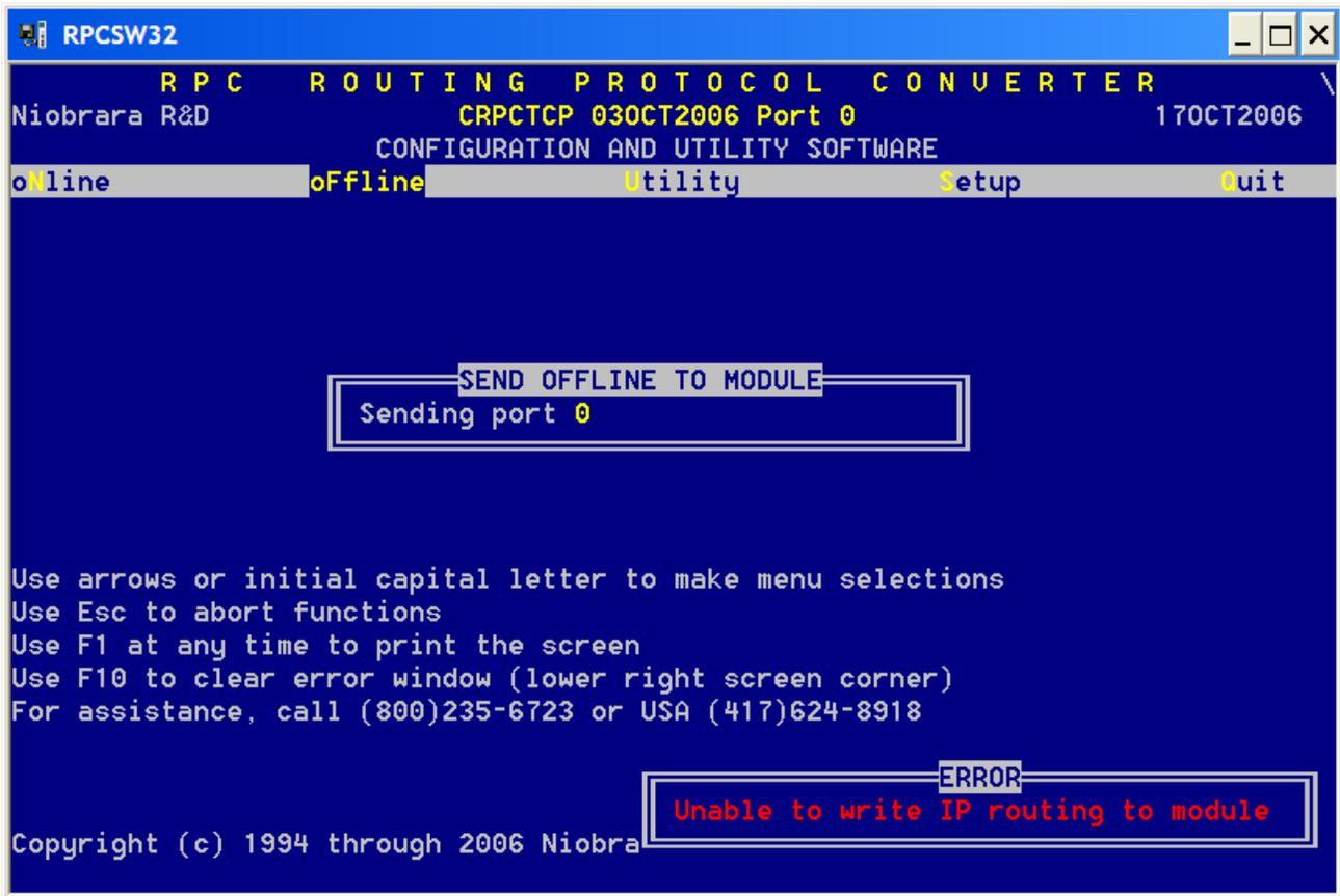
Figure 13: Error received on Send memory to module.
