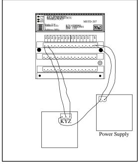
Figure 3 KYZ Wiring Example
