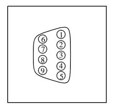
Figure 4-1 InterBus-S Remote Bus In Connector Pinout
