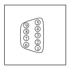
Figure 4-2 InterBus-S Remote Bus Out Connector Pinout
