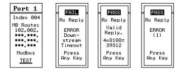
Figure 4.2 Modbus Route Edit TEST Screens
