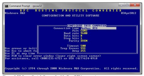
Figure 9.22 Setup Serial Screen for Modbus RTU connection
