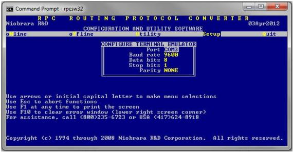
Figure 9.23 Setup Terminal emulator connection
