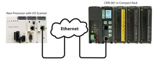
Figure 1: Control Compact Rack with Modbus/TCP I/O Scanner
